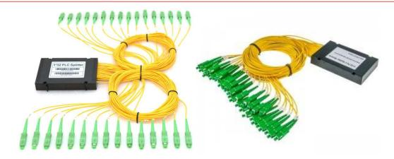
The PLC Splitters is branching devices that is used to distribute optical signals to multiple locations for processing. In optical networks, it is often necessary to split an optical signal into many identical signals, or to combine many signals into a single signal.
